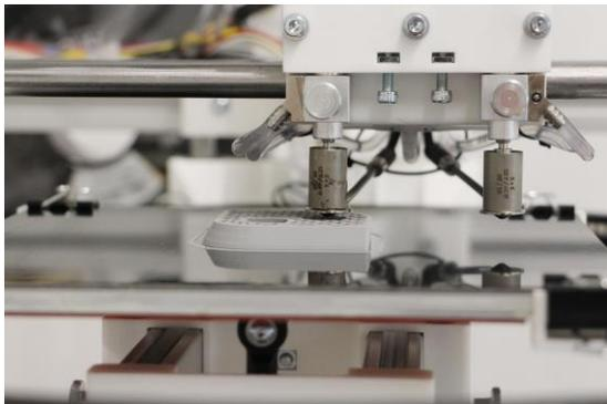
Fused Deposition Modeling (FDM): In this 3D printing process, plastic components are built up layer by layer. (Photo: IPH)
