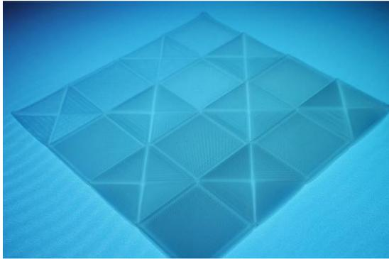
3D-printed sample component: The so-called transmissivity, i.e. light transmission, varies depending on the layer thickness and layer orientation. (Photo: LZH)
