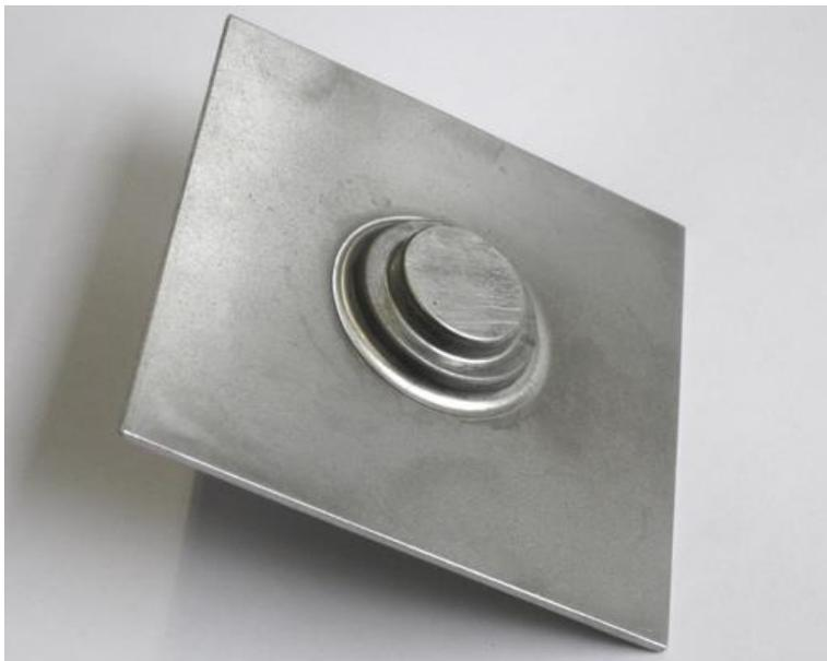
Hybrid compound forging: The novel lightweight production process firmly bonds bulk aluminium parts to steel sheets – already during the forming process without an extra joining step. (Photo: IPH)
