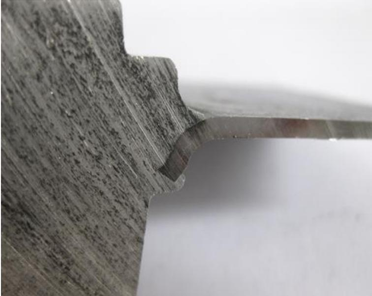
Aluminium stud meets steel sheet: IPH researchers have already succeeded in creating a form-fit connection. Now they want to realize a material bond between the two parts. (Photo: IPH)
