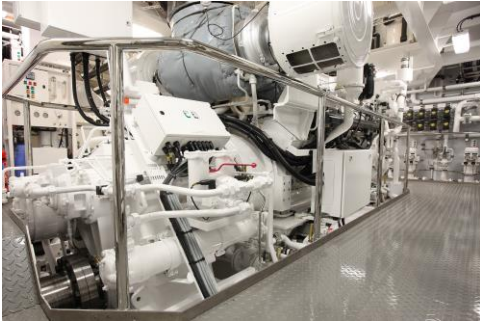
Core of the marine propulsion system: the gearbox. A similar model will be shown at HANNOVER MESSE 2015 to illustrate the new measuring system. (Source: REINTJES GmbH)
