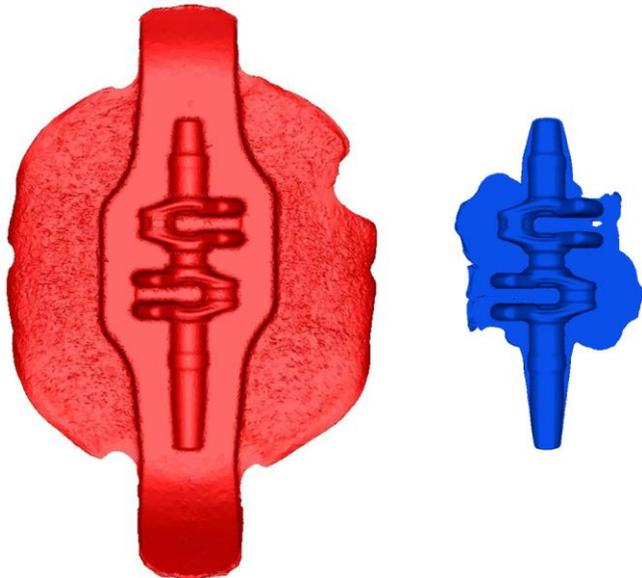
Significantly lower burr percentage: The multi-directionally forged crankshaft (right) compared with a conventionally forged one. (Graphics: IPH)
