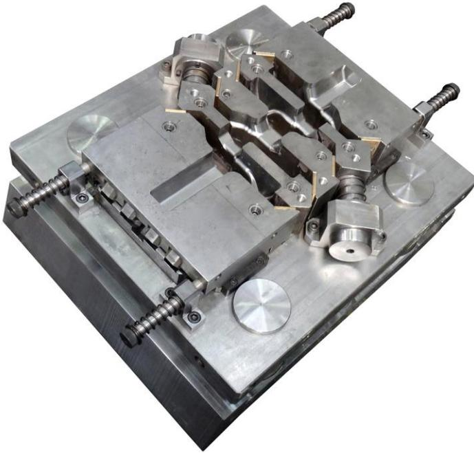
The multi-directional forging tool not only presses metal into the form from above but also at the same time from the sides. This creates fewer burrs. (Photo: IPH)
