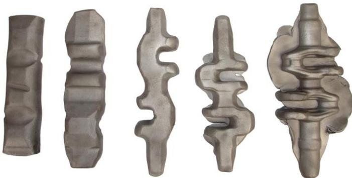
Five forging steps are needed for the finished crankshaft. The fourth step takes place with the multi-directional tool. (Photos: IPH)
