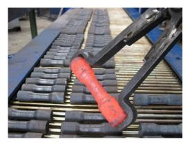
Forged preforms created by using cross wedge rolling must be further processed in order to obtain the final shape.
