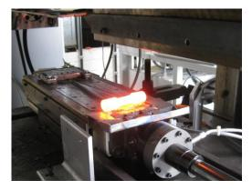
Cross wedge rolling in action at the Institut für Integrierte Produktion Hannover (IPH): As part of the research project "CoVaForm" a similar machine will be constructed and built, especially designed for titanium hip implants.
