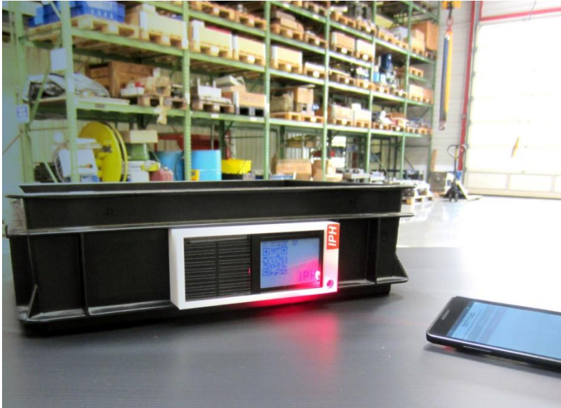
Picture 1: An optical signal with a wavelength of 660 nanometers enables the new label and smartphones to communicate. (Source: IPH)
