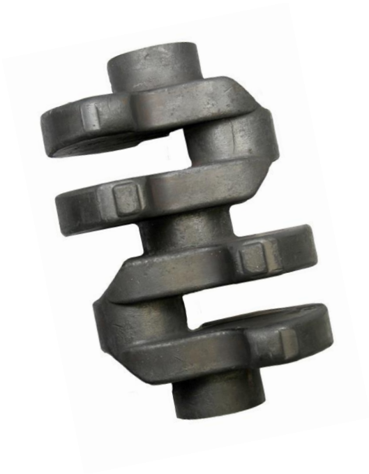
Picture 1: Two-cylinder crankshafts are used in cars and motor-cycles. IPH engineers are trying to produce them using less material. (source: IPH)
