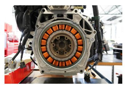
A look inside an electric motor: The narrow air gap between the rotor and stator has a significant impact on efficiency and service life.
