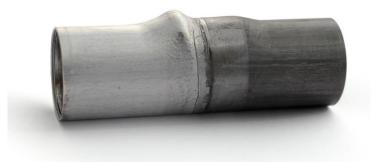
Successful forming experiment: The tube is half made of aluminum, half of steel. The laser-brazed joint area withstood the hydroforming process. (Source: IPH)
